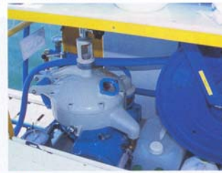
above A large separator uses a centrifugal action to remove water and other contaminants.
