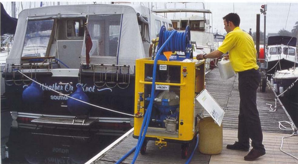
above The Expresslube 'dialysis machine' arrives to clean out a contaminated fuel system.
