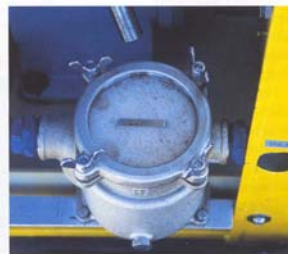
above A pre-filter collects the worst of the contaminants in the circulated fuel.
